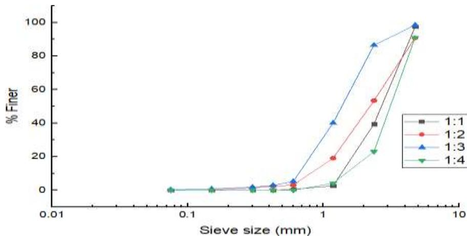
Fig 7 : Sieve analysis of FAPS (12M NaOH and Na<sub>2</sub>SiO<sub>3</sub>)
