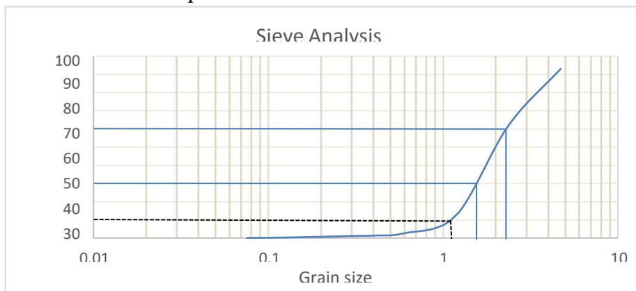
**Fig 3: Sieve analysis of FAPS (6M NaOH and Na<sub>2</sub>SiO<sub>3</sub>)**
