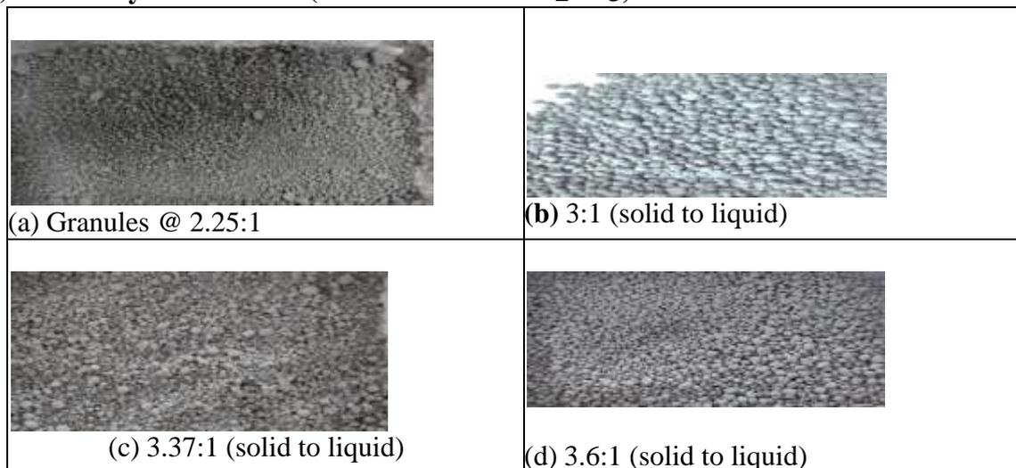
Fig(1): Formation of granules at different fly ash to alkaline solution ratios(a)@2.25:1(b)@3:1 (c) 3.37:1 (d) 3.6:1. These are obtained granules for 10M NaOH solution
