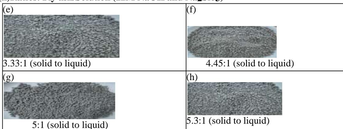
Fig(2): Formation of granules at different fly ash to alkaline solution ratios: (e)@3.33:1 (f)@4.45:1 (g) 5:1 (h) 5.3:1. These are obtained granules for 12M NaOH solution
