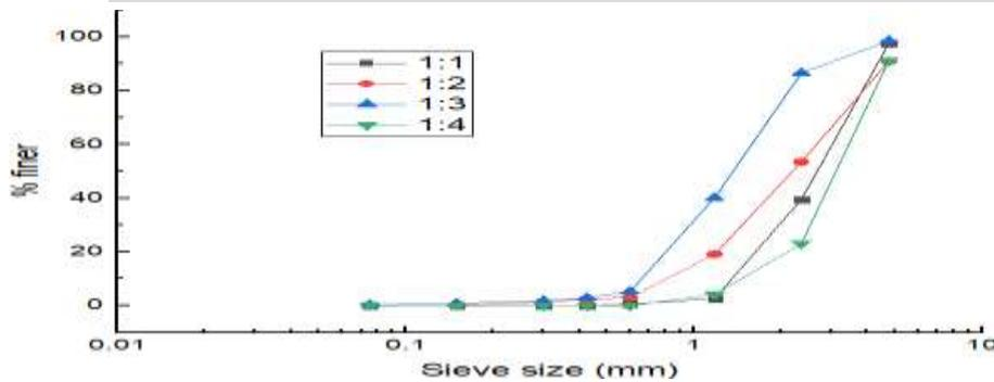
Fig 6: Sieve analysis of FAPS (10M NaOH and Na<sub>2</sub>SiO<sub>3</sub>)
