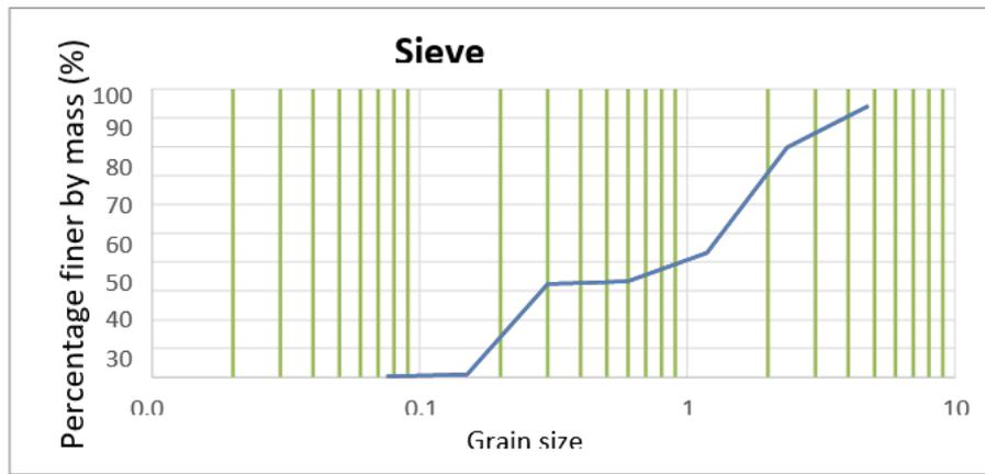
Fig 4: Sieve analysis of FAPS (6M NaOH)
