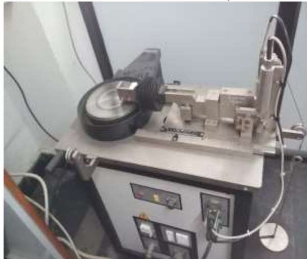
Figure 4: Pin-On Disc set up for wear test
