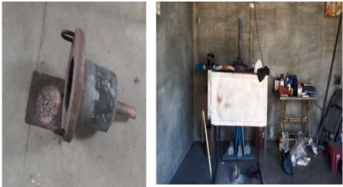
Figure 1: Stir Casting set up
