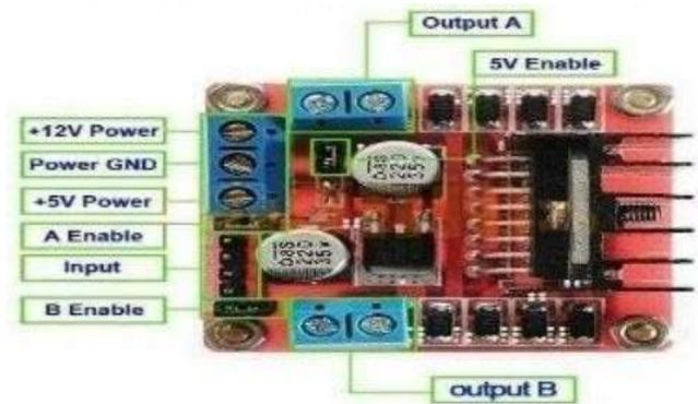
**Fig -6:** Motor drive module diagram
