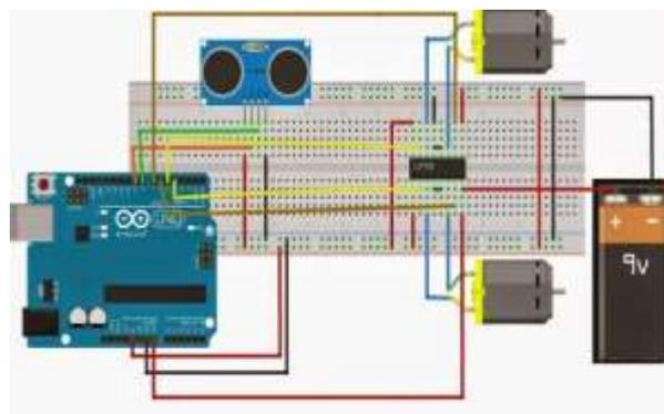
Fig -2:Block diagram of obstacle sensing robot process
