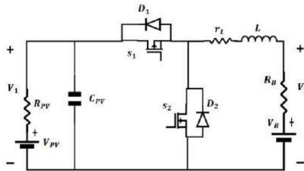
Fig. 2. Bidirectional DC-DC converter.
