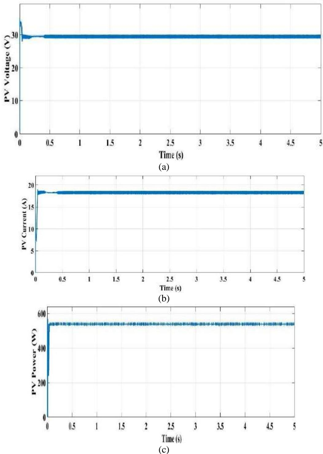
Fig. 6. Solar PV (a) Voltage (b) Current (c) Power at irradiation of  $500 \text{ W/m}^2$ .
