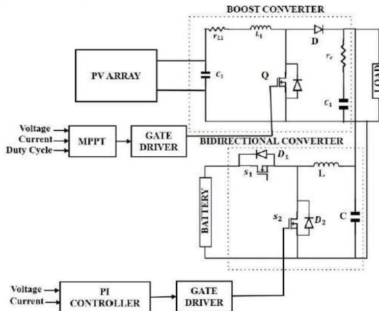
Fig. 1. Schematic diagram of solar PV fed EV.
