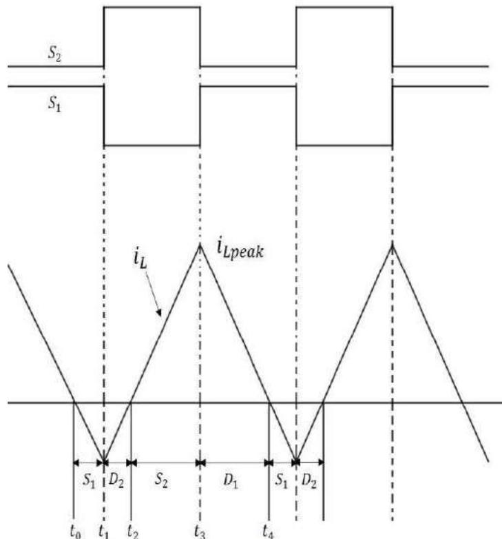
Fig. 3. Gate drivers for switches and diodes.
