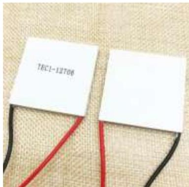
Fig 4: thermoelectric generator
