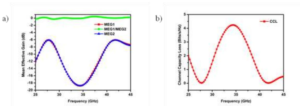
Fig. 6: (a) MEG and (b) CCL simulations for a 2-port MIMO antenna.
