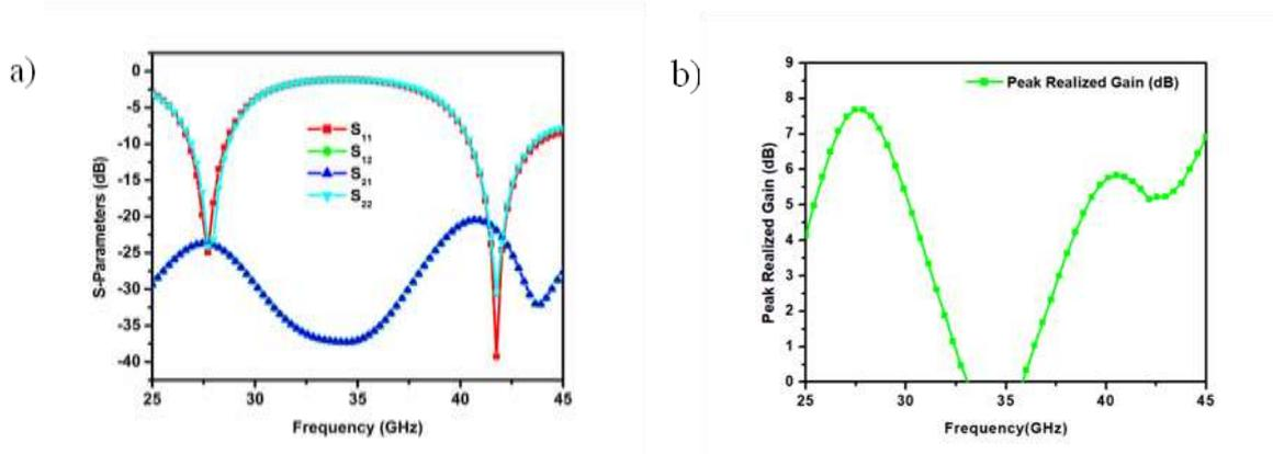
Fig. 4: Stimulated responses of (a) S-parameters and (b) peak realized gain for a 2-port antenna
