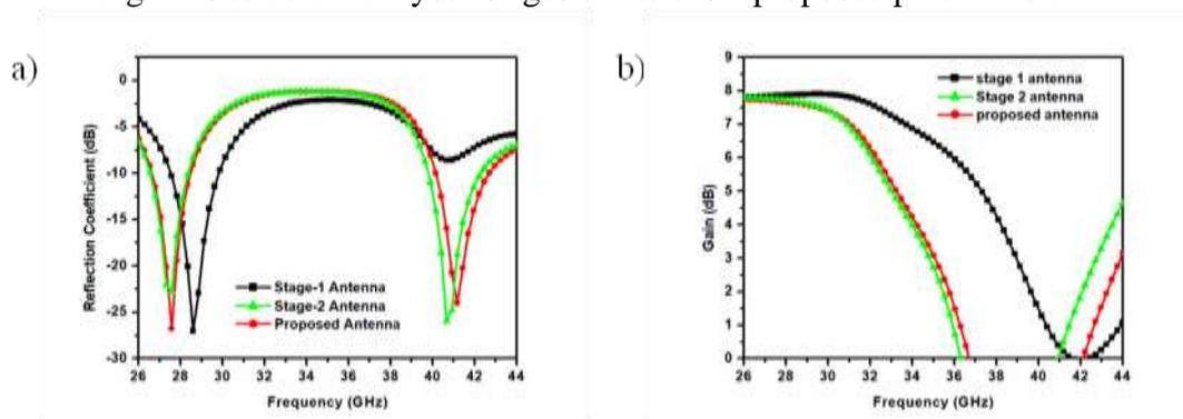
Fig. 2: Simulated response of (a) reflection coefficient and (b) gain of the proposed antenna
