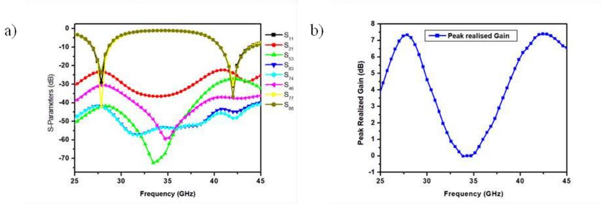
Fig. 9: Simulated response of (a) the S-parameter and (b) the peak realized gain for an 8-port antenna.
