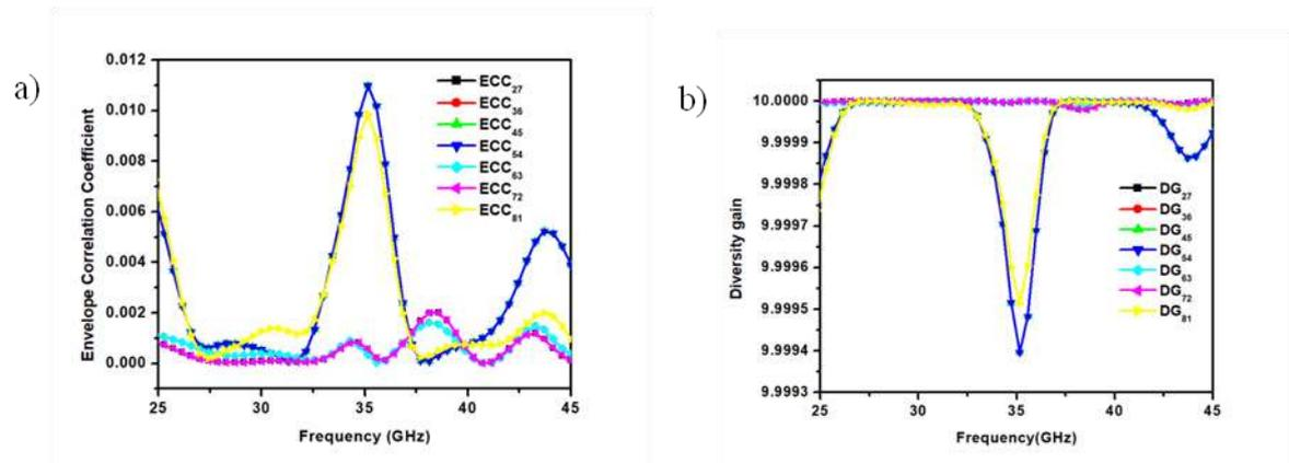
Fig. 10: Simulated 8-port antenna for (a) ECC and (b) DG
