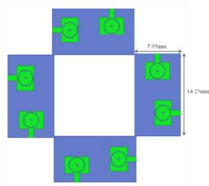
Fig. 8: Geometrical layout for an 8-port MIMO antenna
