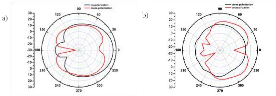
Fig. 7: Simulated E-field Radiation Patterns at (a) 27.85 GHz and (b) 42 GHz
