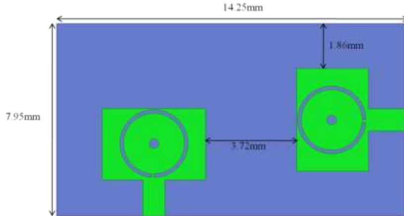
Fig. 3: Geometrical layout for a 2-port MIMO antenna
