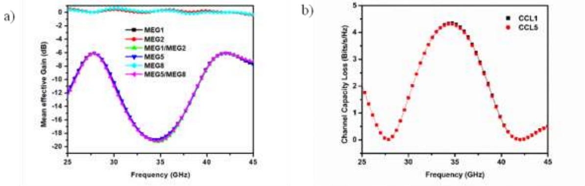
Fig. 11: Simulated (a) MEG, (b) CCL for a 2-port MIMO antenna
