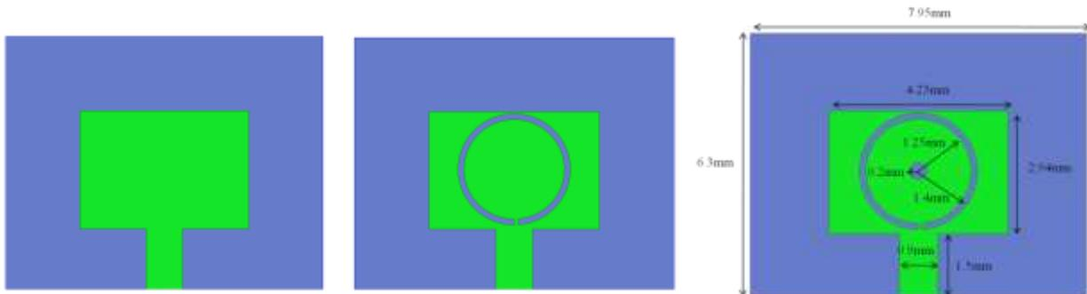
Fig. 1: Geometrical layout stages of the basic proposed patch antenna
