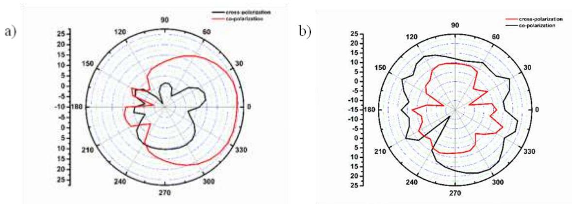
Fig. 12: Simulated E-field Radiation Patterns at (a) 27.85 GHz and (b) 42 GHz
