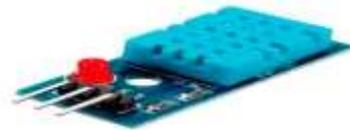
Fig.2 Temperature Sensor
