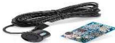
Fig.3 Ultrasonic Proximity Sensor
