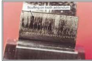
Fig.2- Scuffing on tip of gear tooth
