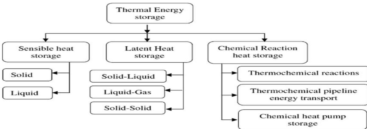
Figure1. A variety of thermal power storage methods
