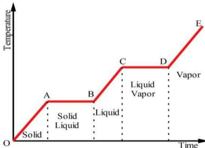
**Graph1:** Time-temperature graph for heating a material
