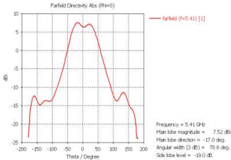
Fig. 3: Simulated 2D radiation pattern of OAM mode l= -1 at 5.41 GHz
