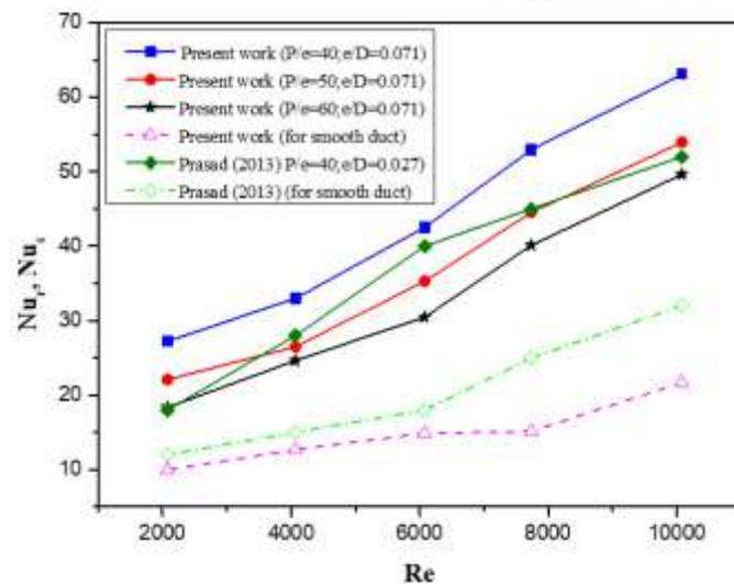
Fig. 4.9 Comparison of effect of P/e on heat transfer in artificially roughened solar air heater
