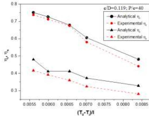
Fig. 4.16 Comparison of analytical and experimental thermal performance of roughened solar air heater at different relative roughness height ( $e/D$ )
