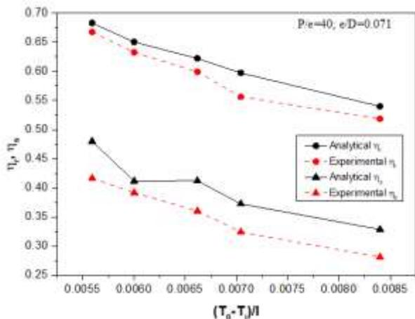
Fig. 4.11 Comparison of analytical and experimental thermal performance of roughened solar air heater at different relative roughness pitch (P/e)
