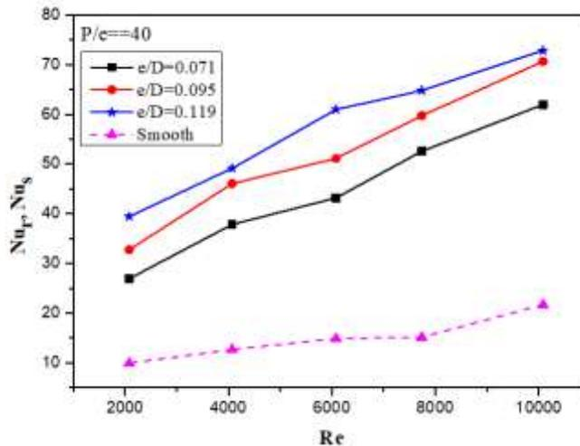
Fig. 4.8 Effect of  $e/D$  on heat transfer in artificially roughened solar air heater
