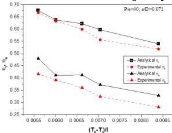
Fig. 4.14 Comparison of analytical and experimental thermal performance of roughened solar air heater at different relative roughness height (e/D)
