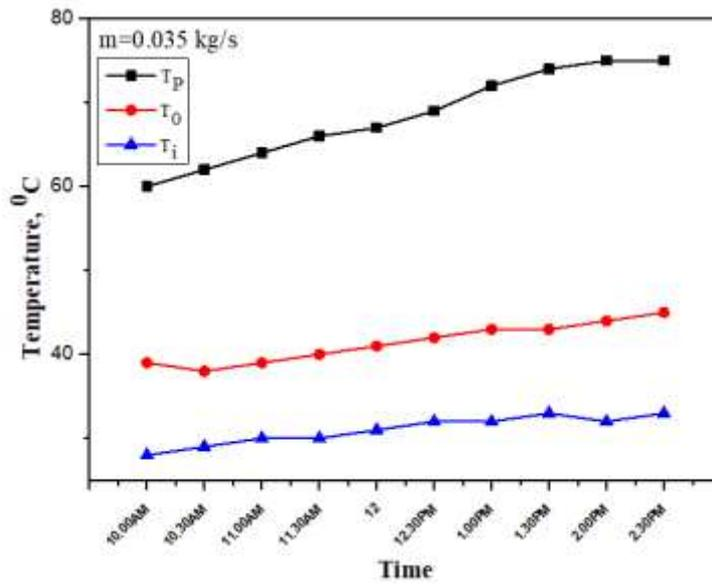
Fig. 4.37 Average hourly variation of  $T_P$ ,  $T_0$  and  $T_i$
