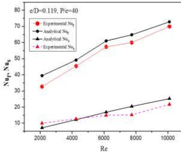
Fig. 4.6 Comparison of analytical and experimental heat transfer data
