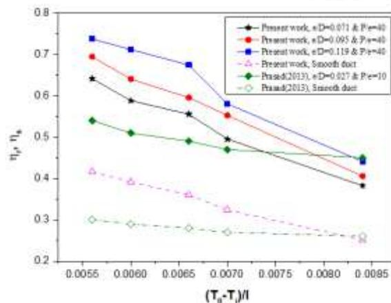
**Fig. 4.20 Comparison of effect of relative roughness height (e/D) on performance of roughened solar air heater**
