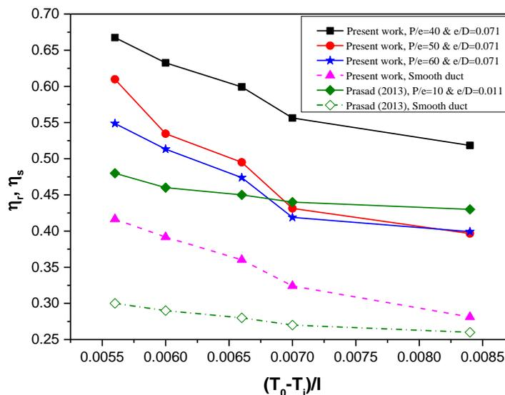
Fig. 4.19 Comparison of effect of relative roughness pitch ( $P/e$ ) on performance of roughened solar air heater
