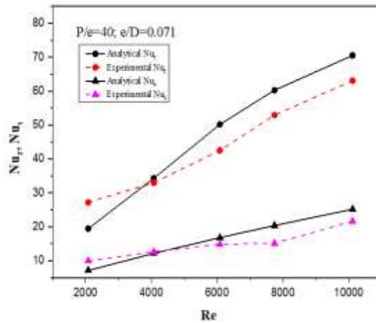
Fig. 4.1 Comparison of analytical and experimental heat transfer data
