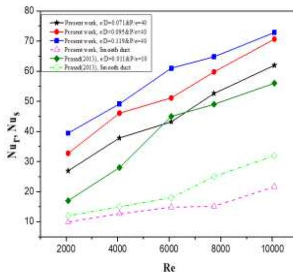
Fig. 4.10 Comparison of Effect of e/D on heat transfer in artificially roughened solar air heater
