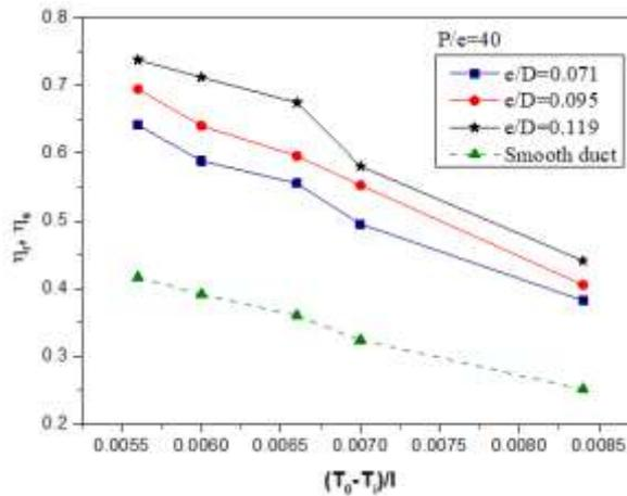
Fig. 4.18 Effect of relative roughness height ( $e/D$ ) on performance of roughened solar air heater
