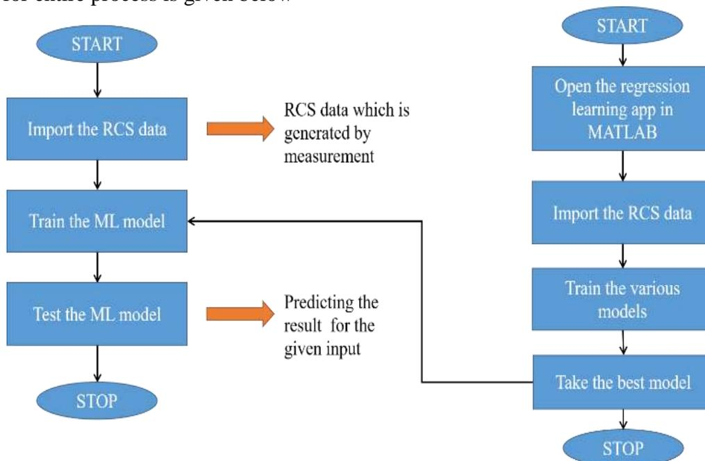
**Fig 1: Flow Chart for Training and Testing**
