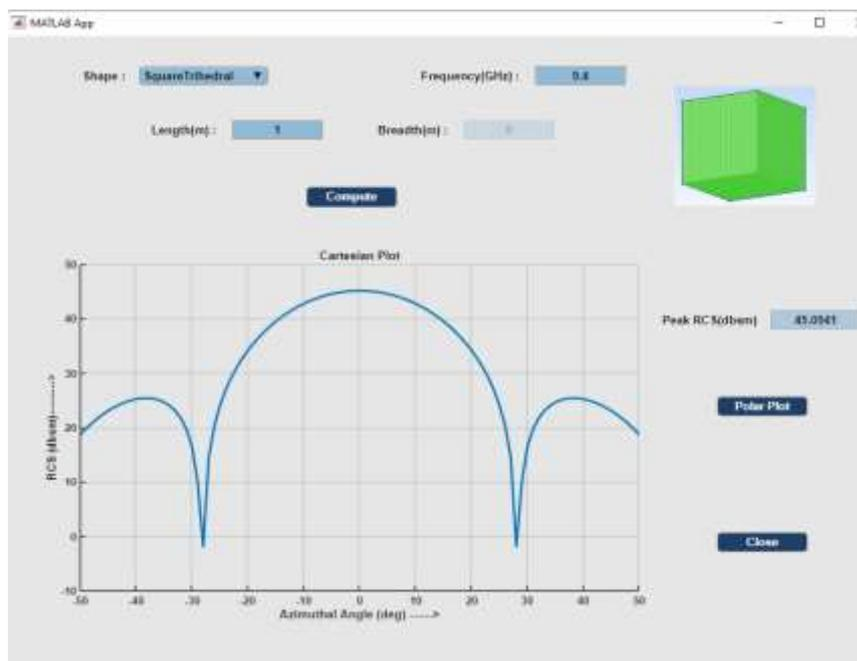
Fig 8 Machine Learning Prediction of RCS for Square Trihedral with side length of 1m at a frequency of 9.4 GHz
