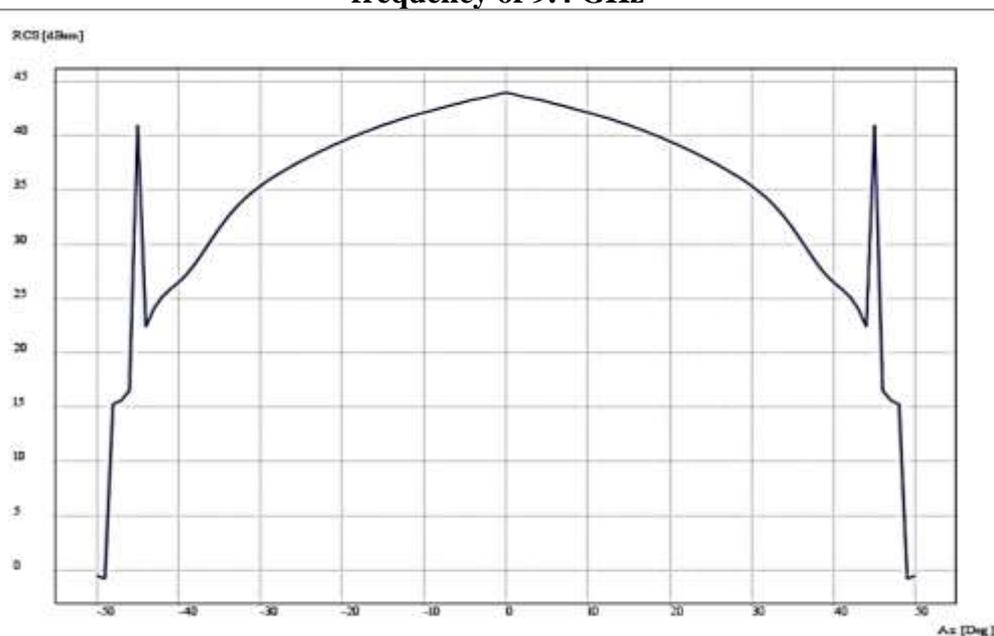
Fig 9 Software based Prediction of RCS for Square Trihedral with length = 1m at a frequency of 9.4GHz
