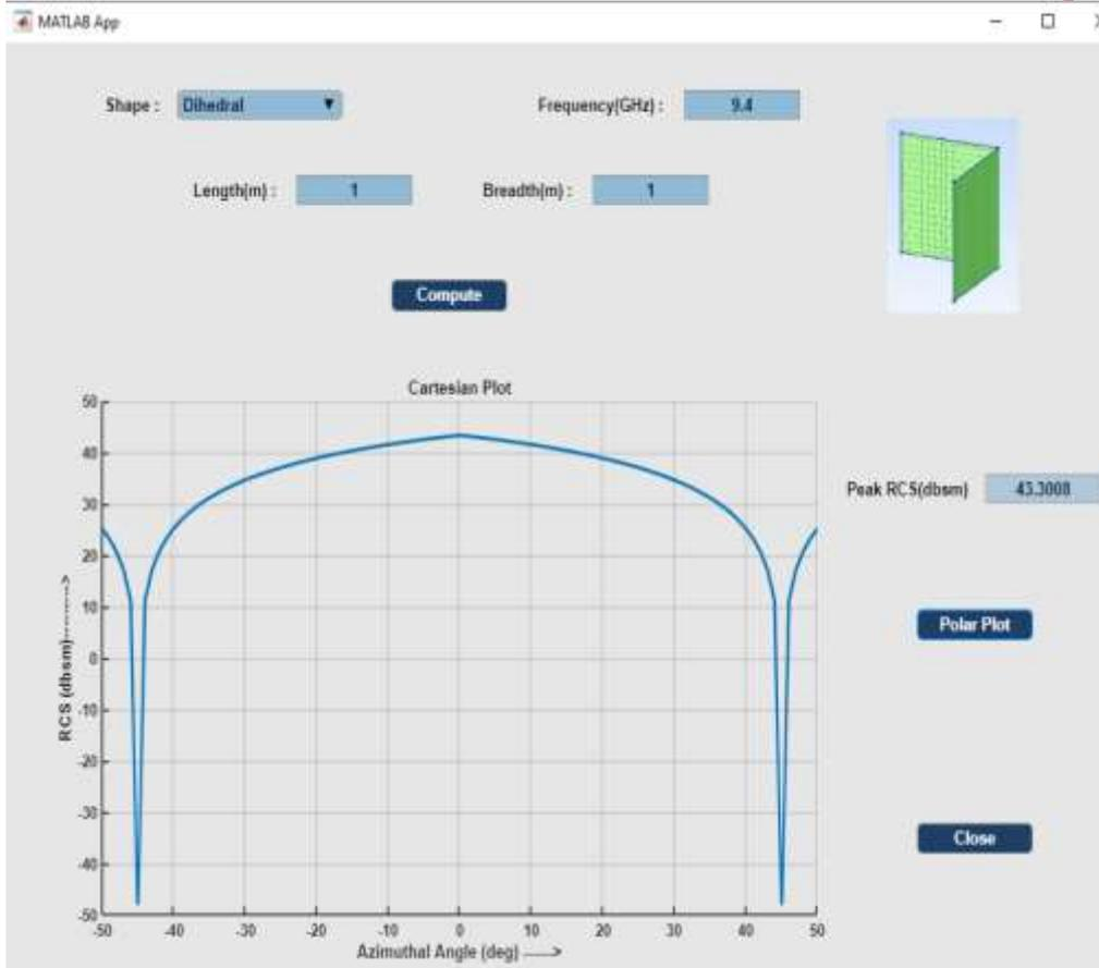
Fig 6 Machine Learning Prediction of RCS for Dihedral with length = 1m and breadth = 1m at a frequency of 9.4 GHz.
