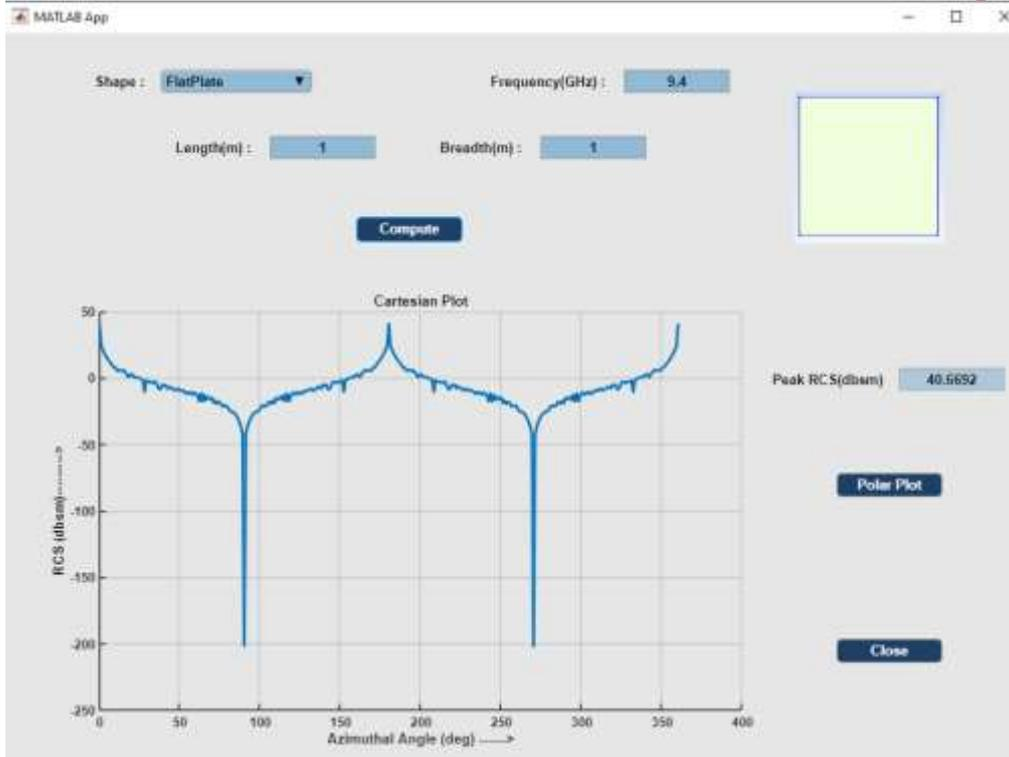
**Fig 3 Machine Learning Prediction of RCS for FLAT PLATE with length = 1m and breadth = 1m at a frequency of 9.4GHz**
