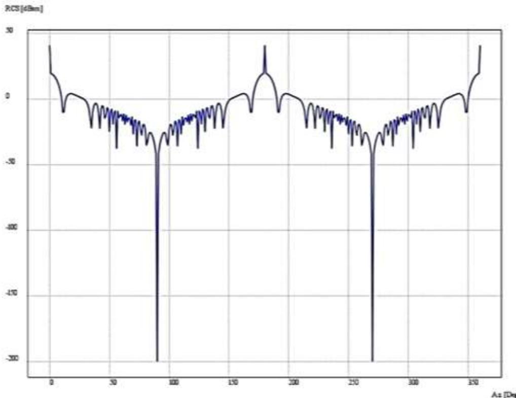
**Fig 4 Software based Prediction of RCS for FLAT PLATE with length = 1m and breadth = 1m at a frequency of 9.4GHz**
