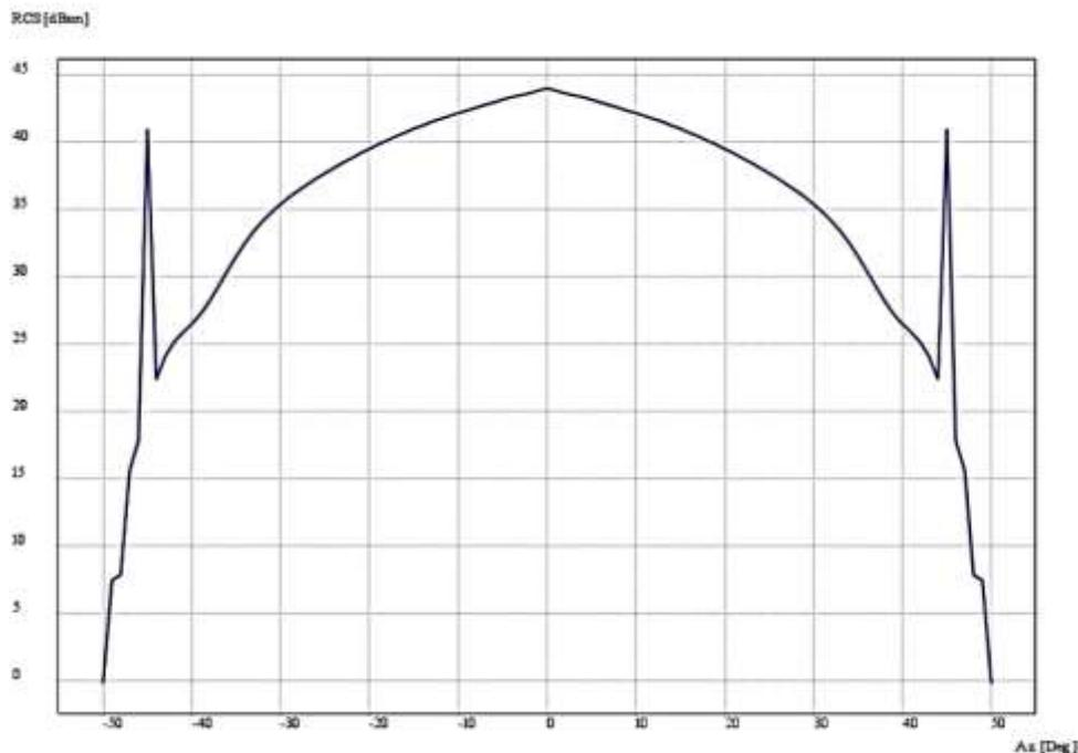
Fig 7 Software based Prediction of RCS for Dihedral with length = 1m and breadth = 1m at a frequency of 9.4GHz
