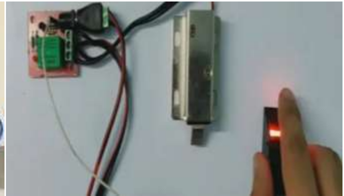
Fig 4: Door Unlocking based on face recognition and fingerprint scanner.
