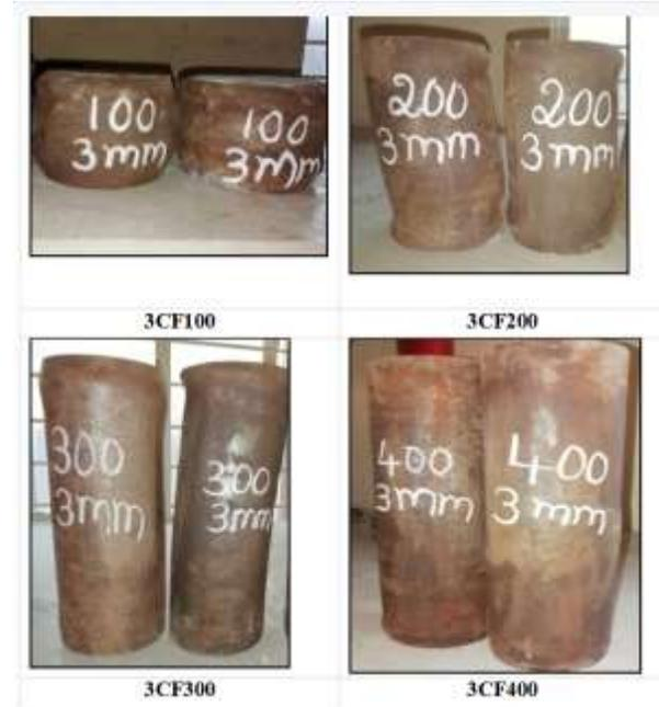
Fig 4.4: Failed specimens of 3mm CFS tubes
