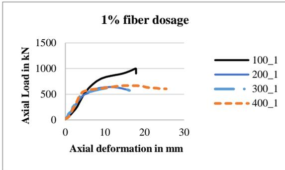
Fig 4.9: Load vs Axial deformation for 1% specimens
