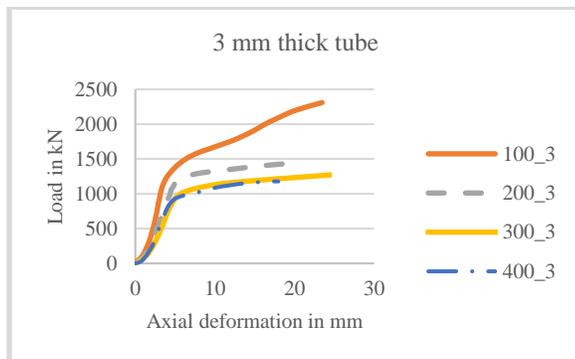
Fig 4.1: Load vs Axial deformation for 3 mm thickness specimen
