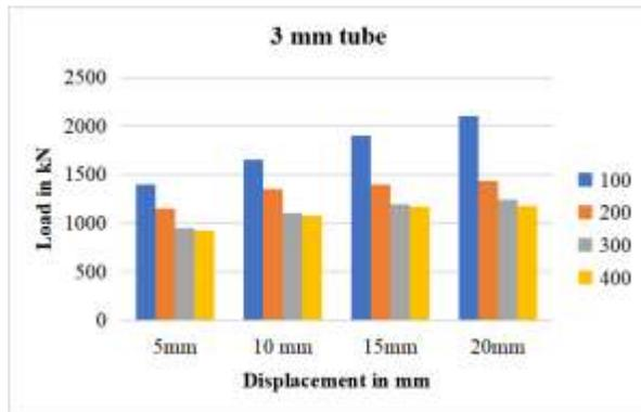
Fig 4.6: Comparison of Load values at different values of displacements in 3mm CFS tube specimens
