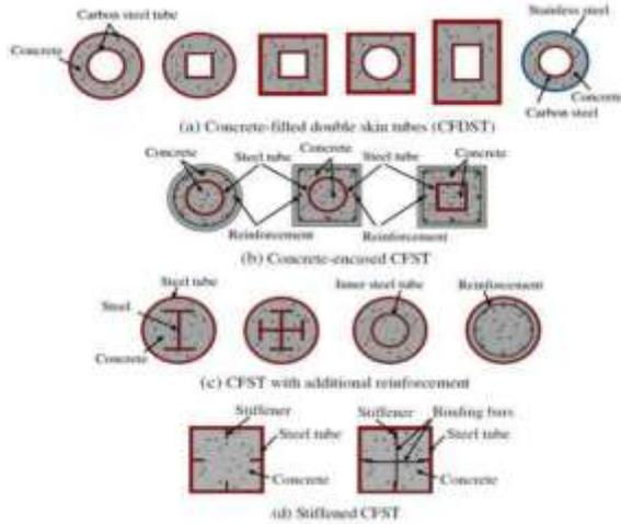
**Fig 1.2: Various types of CFS tube cross sections**
