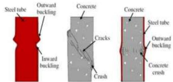
**Fig 1.5: Different failure modes of CFS tube columns**
