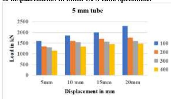
Fig 4.7: Comparison of Load values at different values of displacements in 5mm CFS tube specimens
