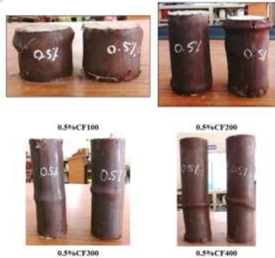
Fig 4.10: Failure modes of 0.5% fiber dosage specimens
