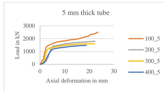
Fig 4.2: Load vs Axial deformation for 5mm thick CFS specimens
