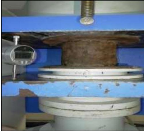
Fig: 3.4 Testing of CFS stub in the first phase of the study
