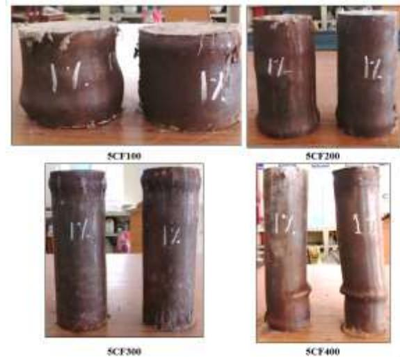
Fig 4.11: Failure modes of 1% fiber dosage specimens
