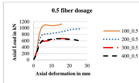
Fig 4.8: Load vs Axial deformation for 0.5% specimens
