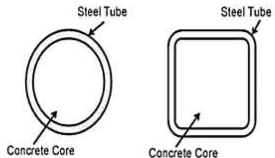
**Fig 1.1: circular and square cross section of CFS tubes**
