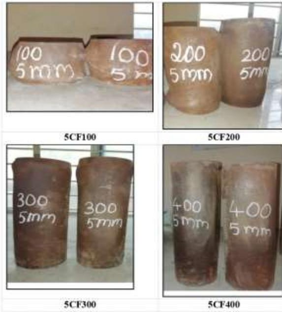
Fig 4.5: Failed specimens of 5mm CFS tubes
