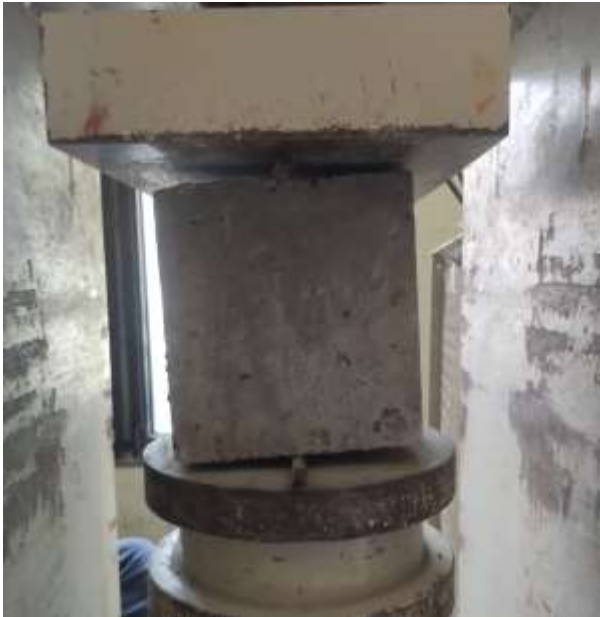
Fig 2.3 Shows the specimen subjecting to pre-cracking
