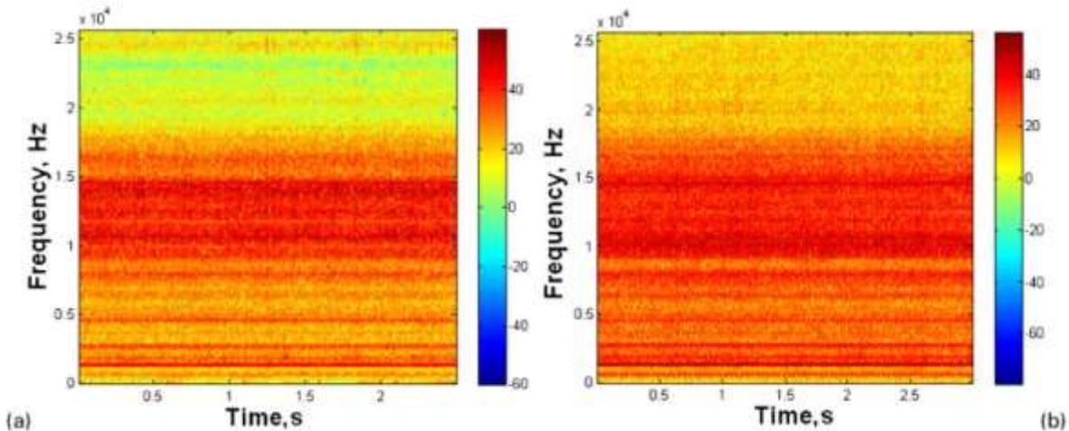
Time- frequency diagrams obtained by using vertical grooved and horizontal grooved pin profiles
