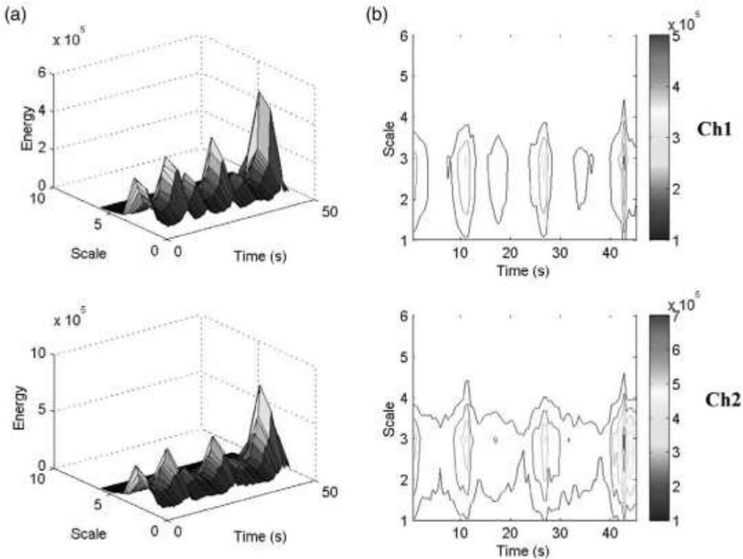
Three-dimensional profile (a) and contour map of wavelet transform (b) for the weld with gap defects.
