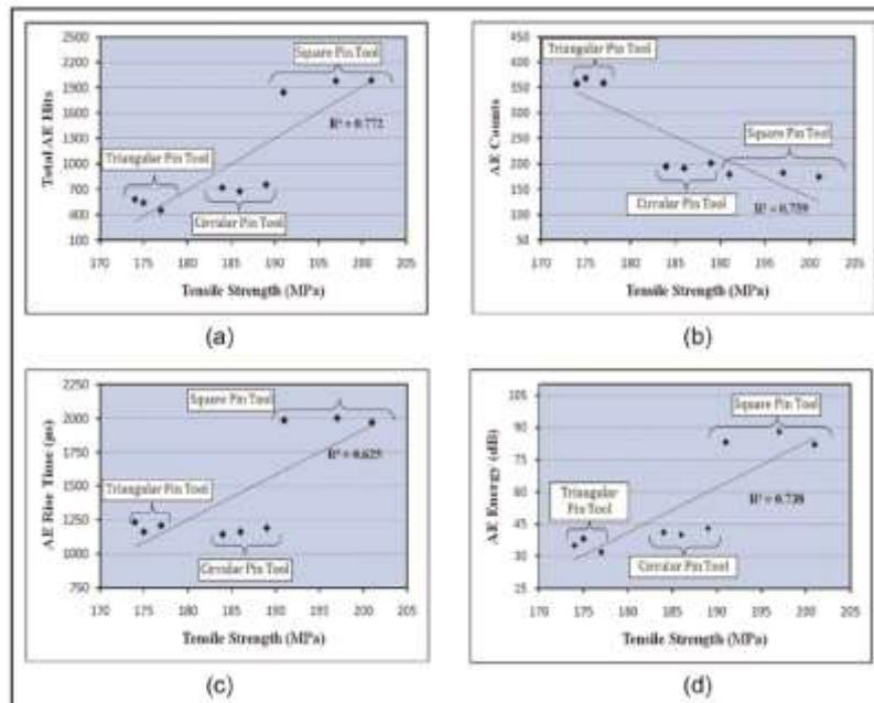
Relationship between AE parameters with tensile strength of FSW specimens produced by different tool pin profiles: (a) AE hits versus tensile strength, (b) AE average counts versus tensile strength, (c) AE rise time versus tensile strength, and (d) AE energy versus tensile strength.
