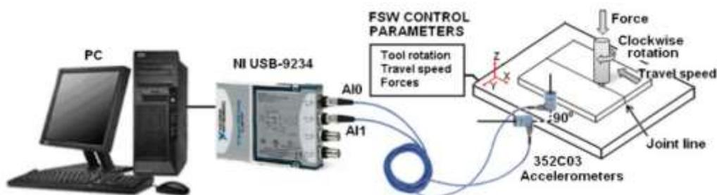
The vibro-acoustical signals of acceleration in Z and Y directions were acquired by using the AE instrument NI USB-9234 connected to PC. The vibro-acoustic signal in the Z axis before tool contact with the workpiece and during welding donot show significant difference in the frequency domain graph. For this reason signals only in the Y axis were analysed.
