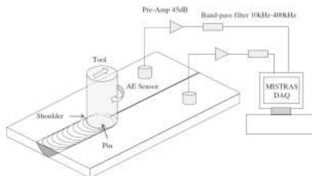
AE signal acquisition, conditioning, and pre-processing
