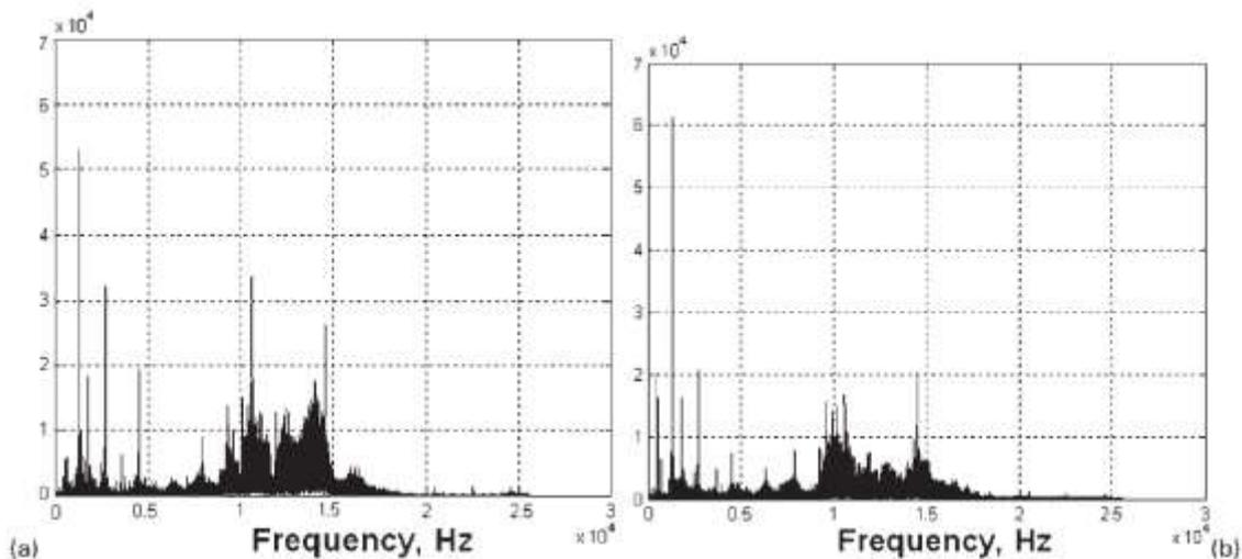
Frequency diagrams obtained by using vertical grooved and horizontal grooved pin profiles.
