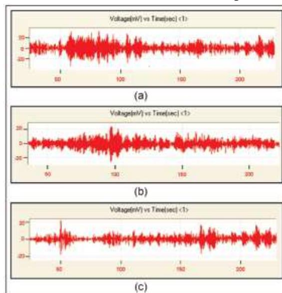
Time-domain AE signal: (a) circular pin, (b) square pin, and (c) triangular pin.
