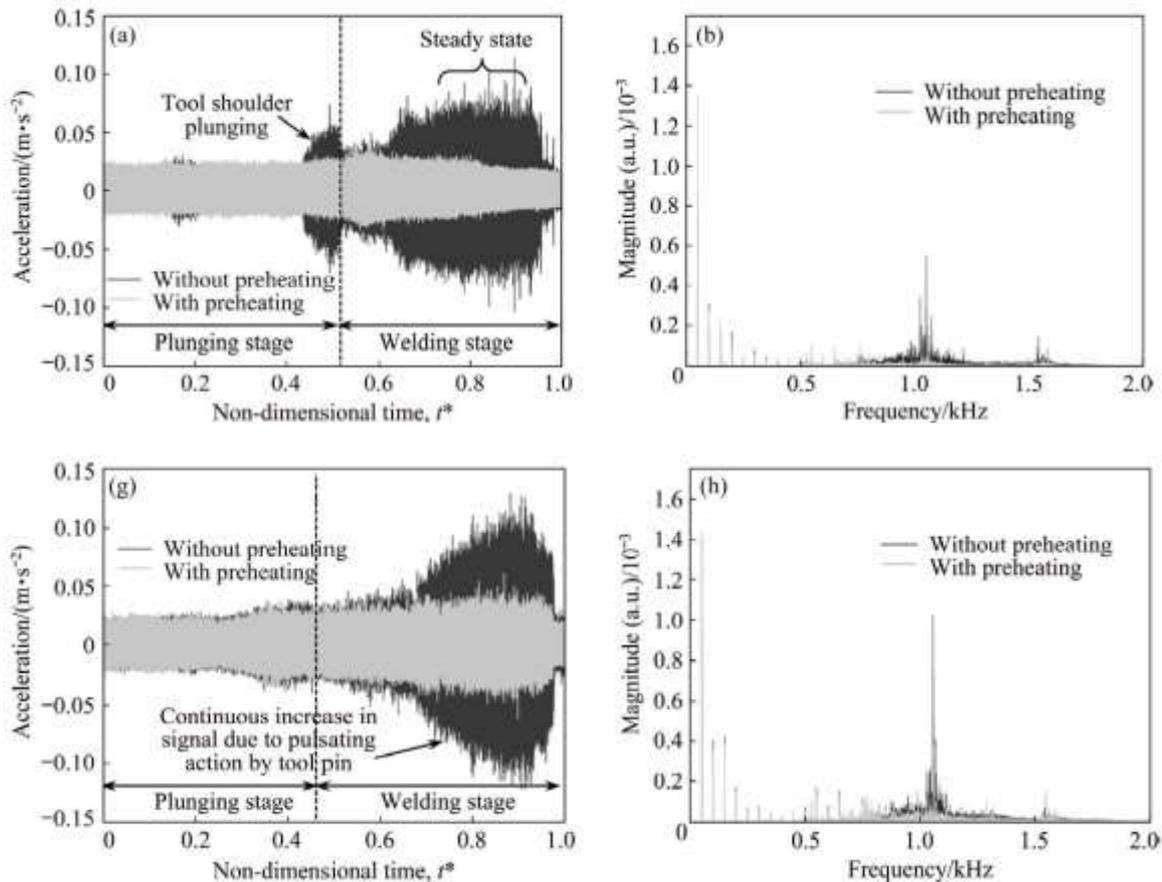
Measured vibro-acoustic signal in time domain (a, g), and converted signal to frequency domain (b, h)
