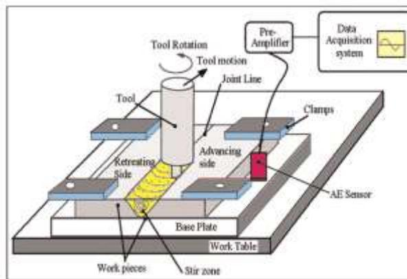
Schematic diagram of experimental setup for friction stir welding
