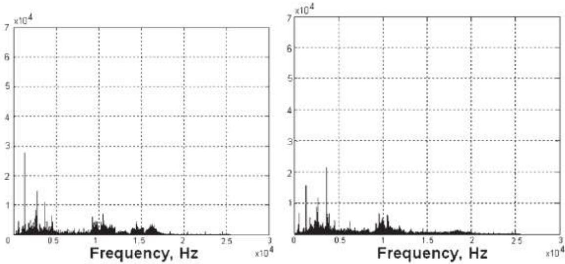
Frequency domain graph before too contact (left) and during welding (right)
