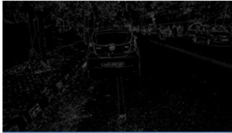
Fig 11. Image frame after canny edge detection
