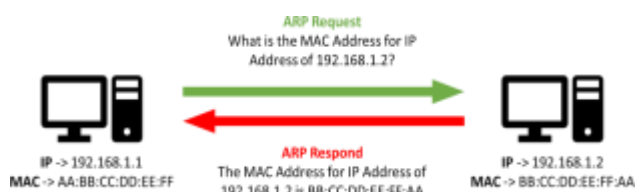
Fig. 2 ARP protocol operation
