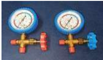
Fig-4: Pressure Gauges
