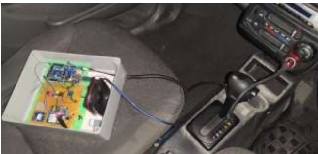
Fig 7. Power supply from CLR to VADS
