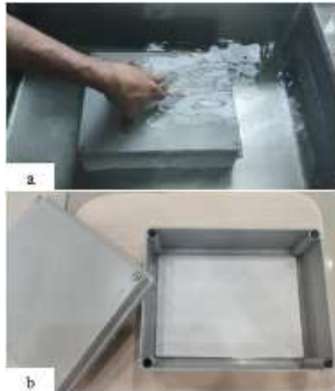
Fig 4. a) Water – resistant test of CPB; b) Interior overlook after water – resistant test
