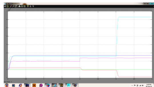
Fig:10. Grid-connected mode Case A-4: the PV-battery system is receiving power from the grid after 2.2 s.
