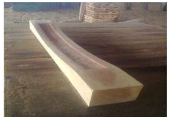
Fig5. Composite leaf spring manufacturing wooden mold.
