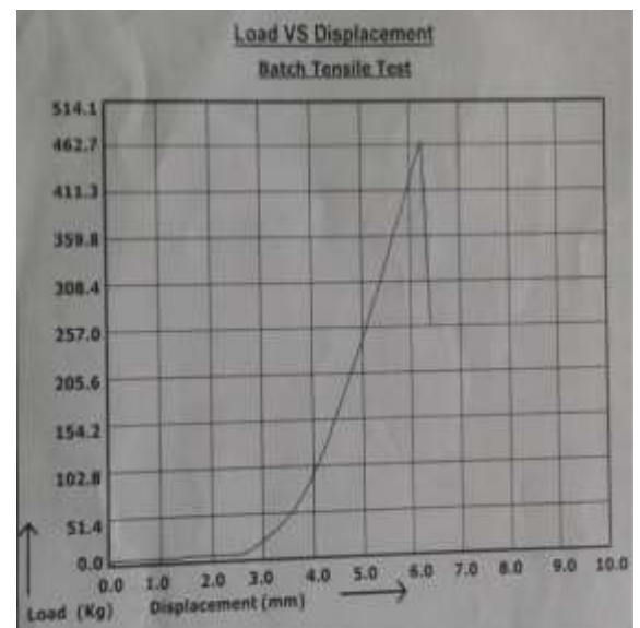
Fig 8. Load vs displacement of polymer matrix leaf spring (E-glass/Vinyl ester/jute).
