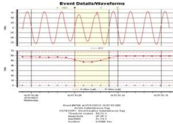
Figure. 6 (a) Field data for balanced voltage sag up to 0.76pu for 0.0398sec.
