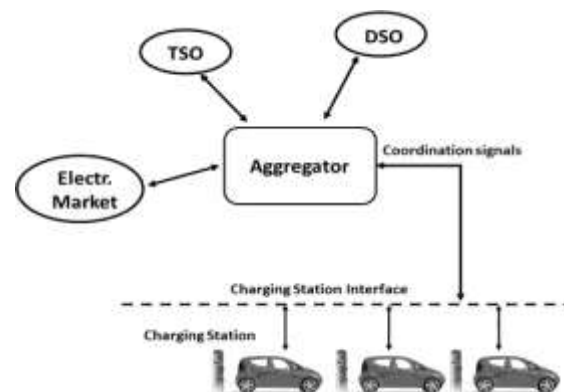
Figure 3. Simplified EV coordination framework: transmission system operator (TSO), distribution system operator (DSO), electric market and charging stations for EVs.
