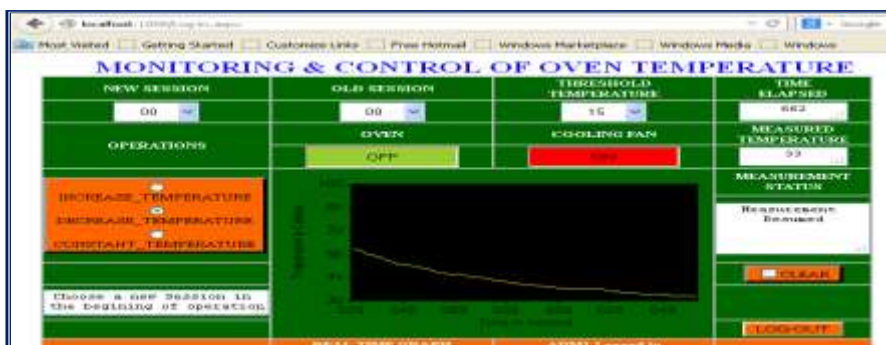
Fig.5.2: Snapshot of DAQ system page-I showing decrease of temperature measured in real time.
