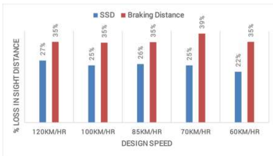
Figure 1: Comparing losses in sight distances for various design speeds at one step below minimum desired design radius
