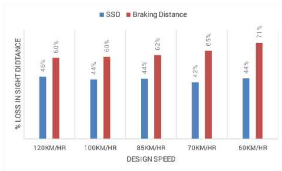
Figure 1: Comparing losses in sight distances for various design speeds at two steps below minimum desired design radius
