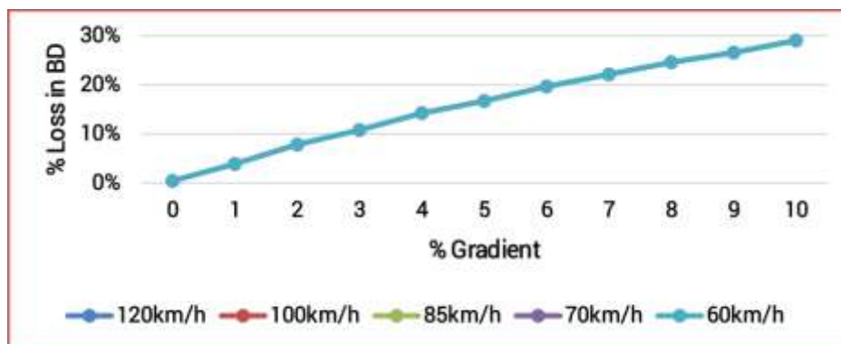
Figure 3: Effect of increasing positive gradient on BDs for various design speeds bands
