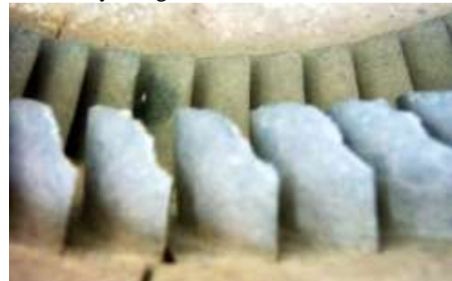
Fig 1.2: Failed Stator Blades
