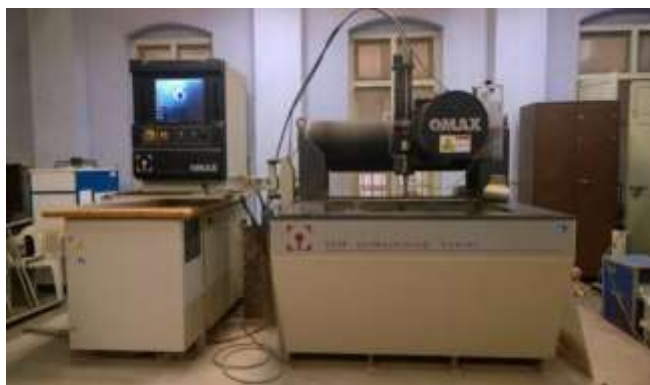
Fig 9: Photograph of AWJ machining setup facility
