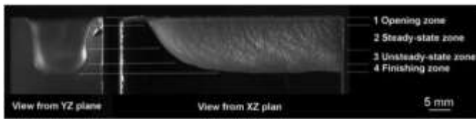
Fig 5: Four erosion zones during the channel formation [9]
