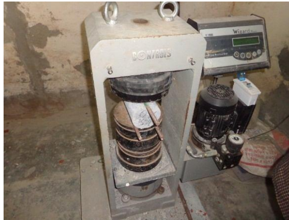
Figure 4: Experimental set-up of splitting tensile strength test
