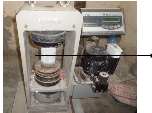
Figure 3: Placement of cylindrical specimen for compressive strength test
