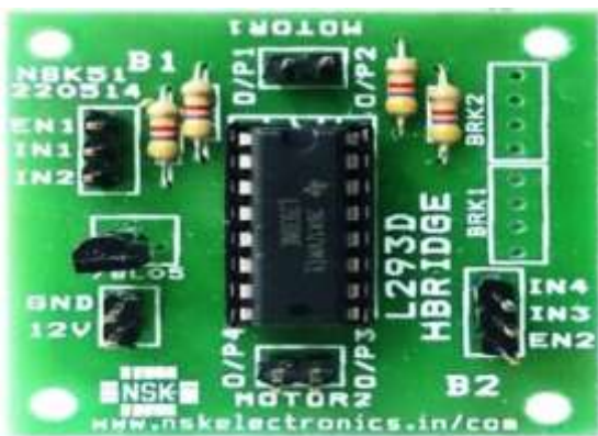
Figure 4 (a). Motor driver circuit of H-bridge
