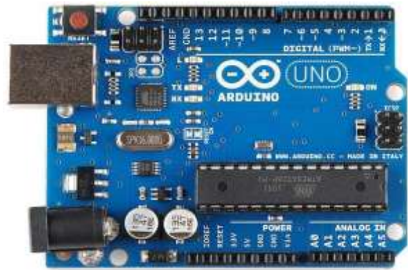
Figure 7. Arduino UNO board
