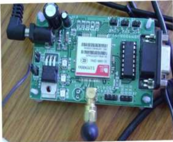
Figure 6. GSM SIM900 Circuit
