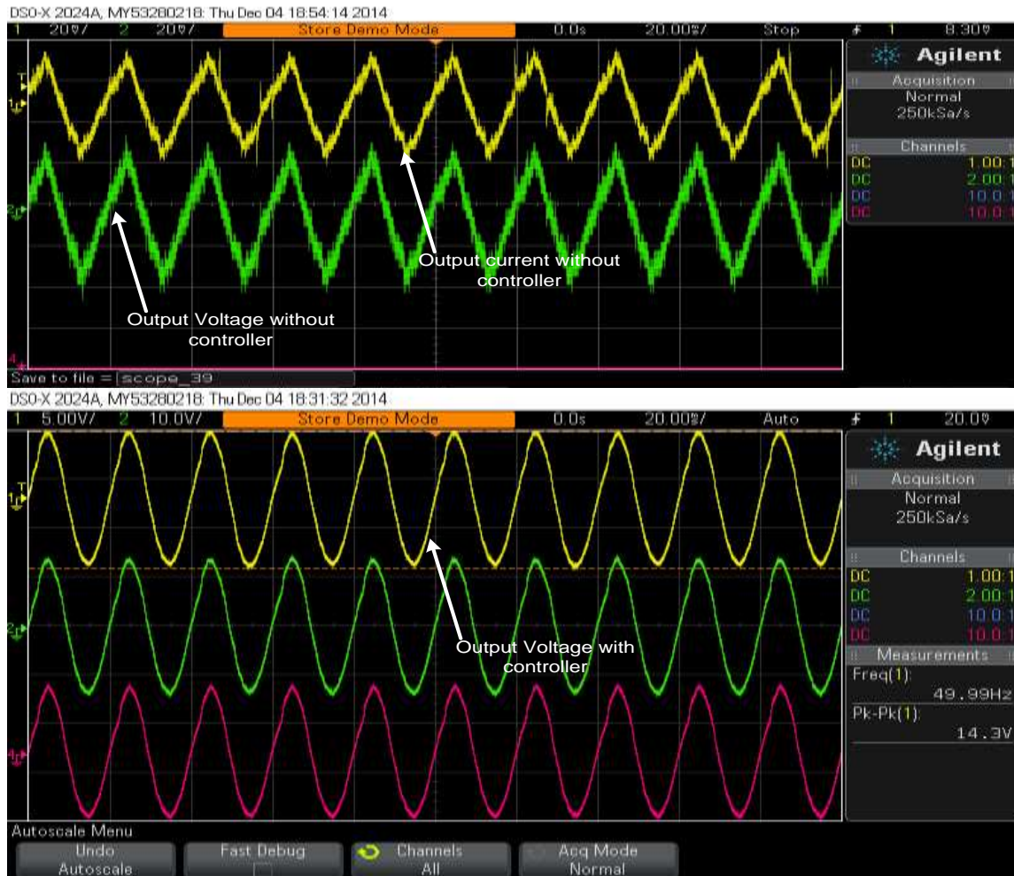
Fig. 10 Experimental results for variable wind speed and constant incremental speed showing its constant voltages.
