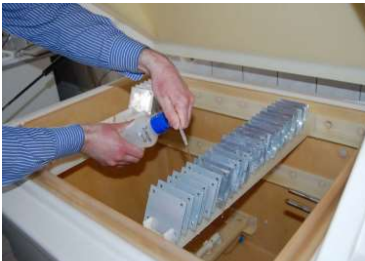
Figure 1. Samples inside salt spray chamber.
