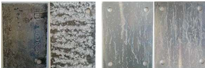
Figure 4. Result of untreated and treated AA7075 alloy with various coating mass (0.16 g/m 2 ) left and (0.36 g/m 2 ) right.
