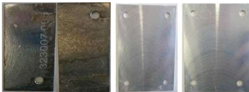
Figure 5. Result of untreated and treated AA6082 alloy with various coating mass ( 0.12 \text{ g/m}^2 ) left and ( 0.46 \text{ g/m}^2 ) right.
