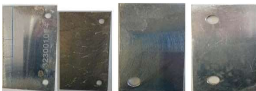
Figure 6. Result of untreated and treated AA6063 alloy with various coating mass ( 0.15 \text{ g/m}^2 ) left and ( 0.3 \text{ g/m}^2 ) right.
