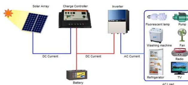
Figure 1. Schematic diagram of a typical Solar Home System.
