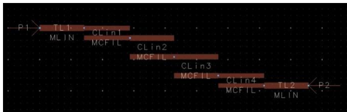
Fig. 7 Layout of parallel-coupled microstrip band pass filter.
