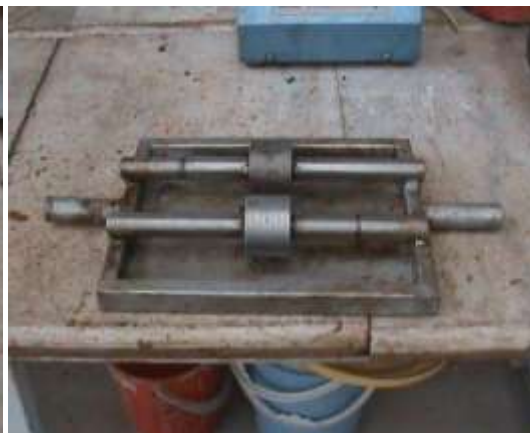
(b) roller for compacting the specimens
