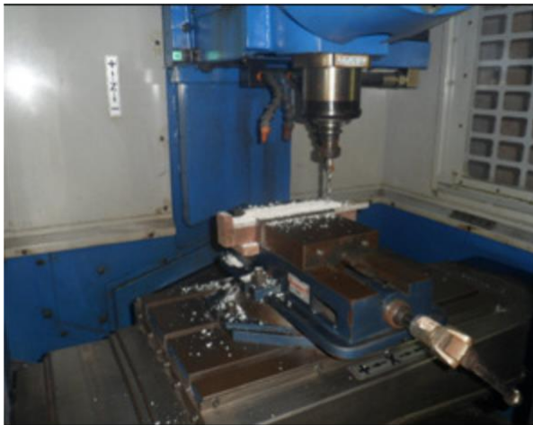
Figure 3 VMC performing drilling on composite laminate and 10mm
