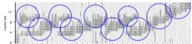
Figure 6: Results of the Attack on the LLC Sets Containing Instructions (AES rounds are marked)
