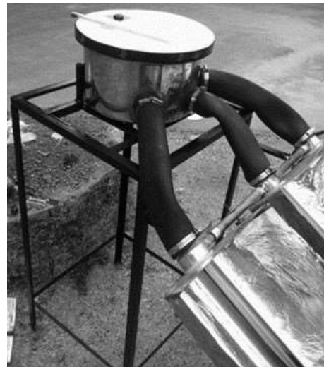
Figure 6: Oil storage tank connected to CPC
