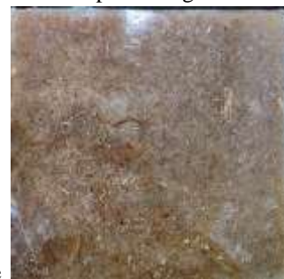
Fig: 184gms Epoxy + 116gm Hardener + 15gm coconut fiber Pictures representing the formation of the composite
