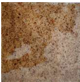
Figure: 184gms Epoxy + 116gm Hardener + 20gm Sugar cane fibbers Pictures representing the formation of the composite
