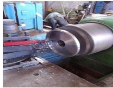
Figure 5 casing disk during manufacturing
