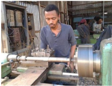
Figure 4 Shaft during manufacturing
