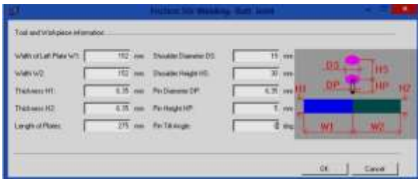
Fig.4 Tool & workpiece information input in HyperWeld.
