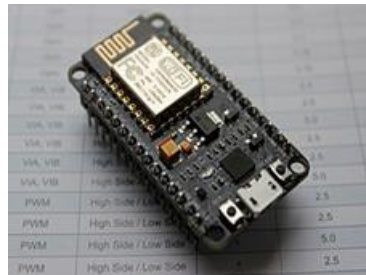
Fig.(8) : Node MCU board
